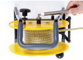
Figure 2 To Test the Entire System: Make sure sensitivity dial is turned fully clockwise. Touch the probe body to the standoff screw and probe tip to the stud (on axle) at the same time. The buzzer will sound if the system is okay.
