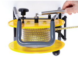
Figure 2 To Test the Entire System: Make sure sensitivity dial is turned fully clockwise. Touch the probe body to the standoff screw and probe tip to the stud (on axle) at the same time. The buzzer will sound if the system is okay.
